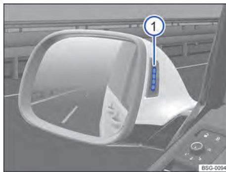
Fig. 125 In the exterior mirror housing: visual displays of Blind Spot Assist.
