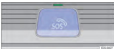
Fig. 51 In the roof console: button for eCall Emergency System (behind button cover) and indicator lamp.
