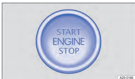
Fig. 105 In the lower section of the centre console: starter button for starting the engine.
