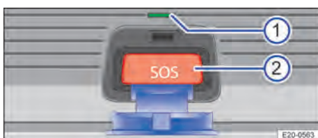
Fig. 52 Control for emergency call: indicator lamp and button for eCall Emergency System.
