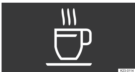
Fig. 15 On the instrument cluster display: Drowsiness Monitor symbol.
