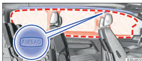
Fig. 37 On the left-hand side of the vehicle: location and deployment zone of the curtain airbag (7-seater).
