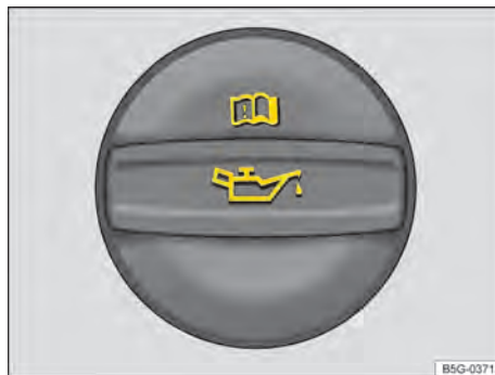
Fig. 209 In the bonnet space: cap of engine oil filler opening (illustration).
