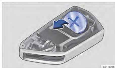
Fig. 56 Vehicle key: changing the button cell.
