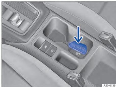
Fig. 106 In the centre console: emergency start function.
