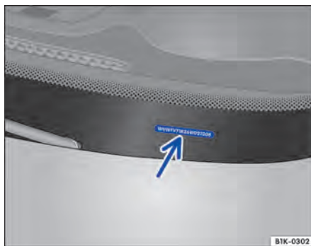
Fig. 275 In the windscreen: vehicle identification number.
