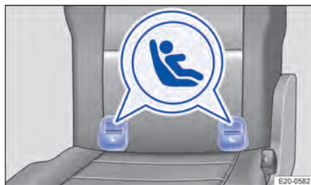
Fig. 43 On vehicle seat in third seat row: marking variants identifying the ISOFIX anchorage points for child seats.
