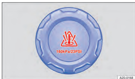
Fig. 212 In the bonnet space: cap of the coolant expansion tank.
