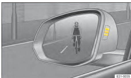
Fig. 127 In the exterior mirror housings: display of the Exit Warning system (illustration).
