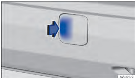
Fig. 201 In the rear bumper on the right: removing the cover.
