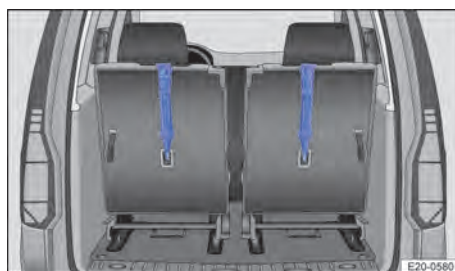
Fig. 48 Third seat row: top tether straps attached in top tether anchor point (depending on equipment).
