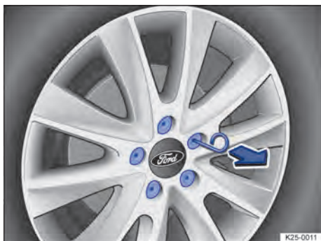
Fig. 226 Removing caps from the wheel bolts with the hook (illustration).
