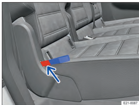
Fig. 70 Second row of seats: marking indicating that the seat backrest is not engaged properly.
