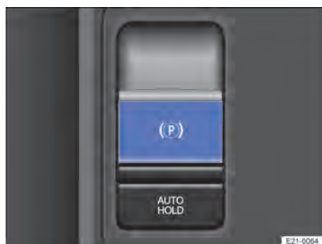
Fig. 126 In the centre console: button for the electric parking brake.
