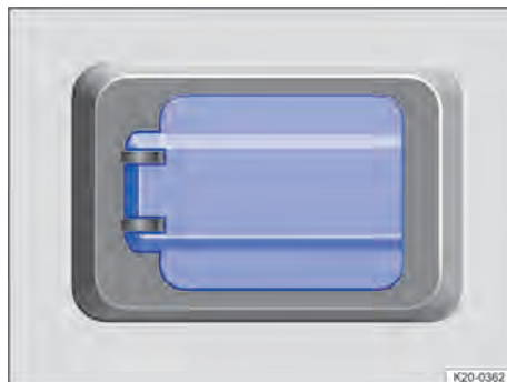
Fig. 144 On the rear centre console or on the partition to the load compartment: 230-volt socket with earthing contact with cover flap (illustration).
