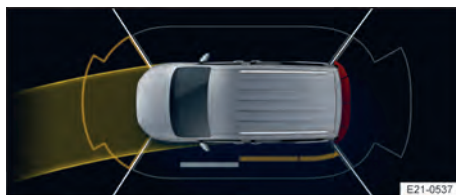
Fig. 129 On the Infotainment system: obstacle detection and steering wheel angle for Parking Sensors (illustration).
