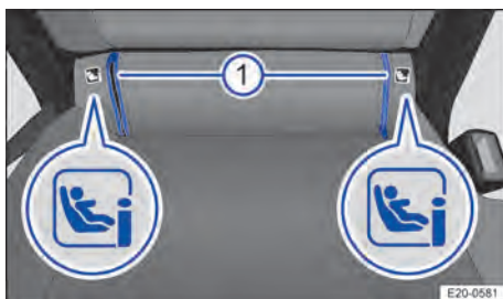
Fig. 42 On vehicle seat in second seat row: marking variants identifying the ISOFIX anchorage points for child seats.
