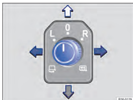
Fig. 97 In the driver door: rotary knob for the exterior mirrors
