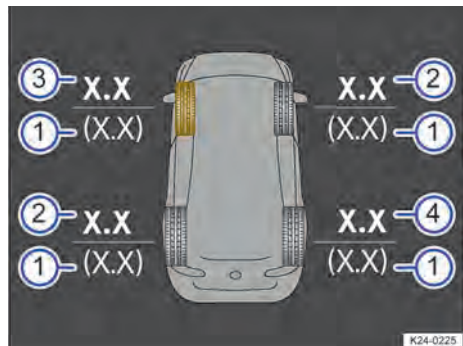
Fig. 220 Display in the Infotainment system: current tyre pressures (illustration).
