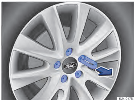
Fig. 225 Removing caps from the wheel bolts with the puller (illustration).
