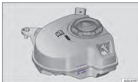
Fig. 213 In the bonnet space: marking on the coolant expansion tank (illustration).
