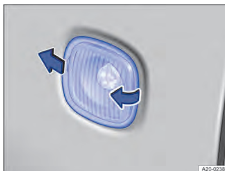
Fig. 184 On the side of the vehicle: removing the direction indicator repeater.
