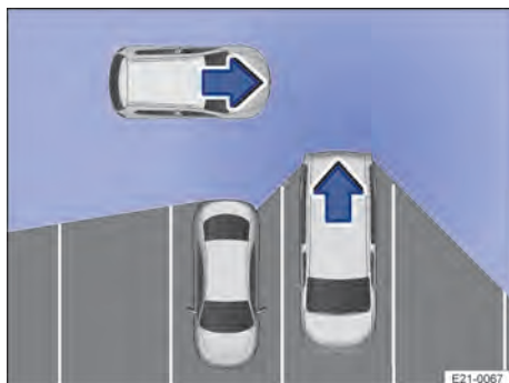
Fig. 138 Illustration of Cross Traffic Alert: monitored area around the vehicle leaving the parking space.
