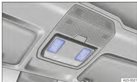
Fig. 91 In the roof console: touch-sensitive reading lights.
