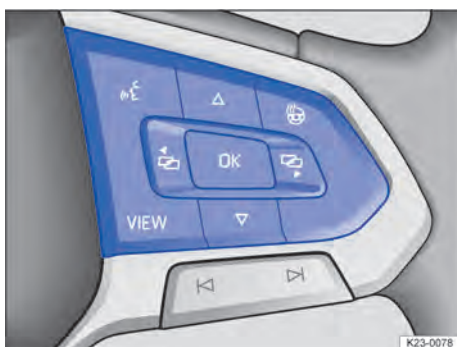
Fig. 11 Right side of the multifunction steering wheel: operating the digital instrument cluster Pro (illustration).
