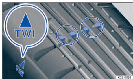
Fig. 219 In the tread grooves: tread wear indicators.
