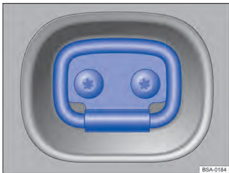
Fig. 161 In the load compartment: fastening rings.
