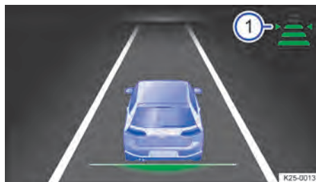
Fig. 120 On the display of the digital instrument cluster: set distance ①, Adaptive Cruise Control is controlling the vehicle (illustration).
