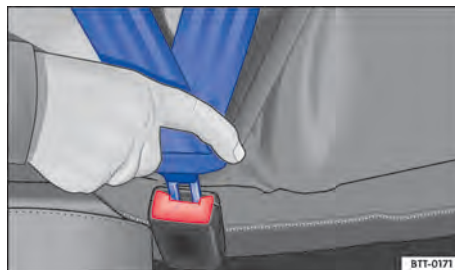
Fig. 23 Inserting the seat belt latch plate into the buckle.
