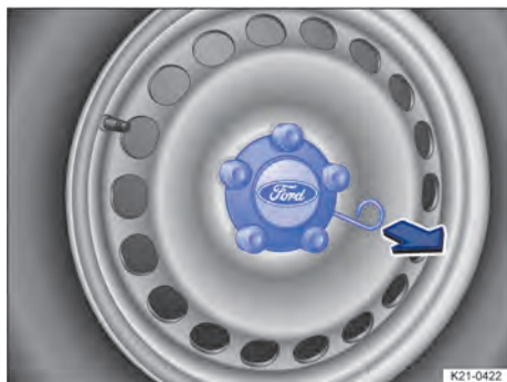
Fig. 223 Pulling off the centre wheel trim (illustration).
