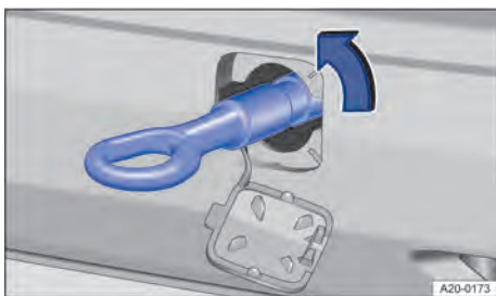
Fig. 202 In the rear bumper on the right: screwing in the towing eye.
