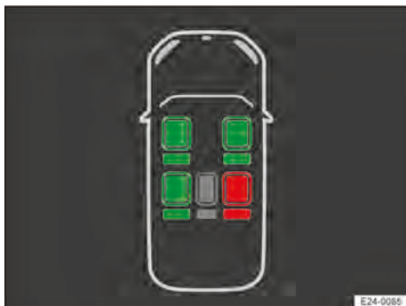
Fig. 22 On the display of the instrument cluster: Seat belt warning system (illustration).
