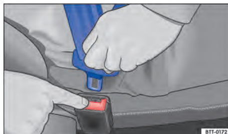
Fig. 24 Removing the latch plate from the buckle
