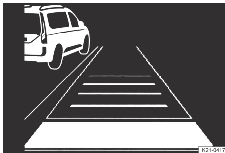
Fig. 117 In the instrument cluster display: slower vehicle detected in the left-hand lane (illustration).
