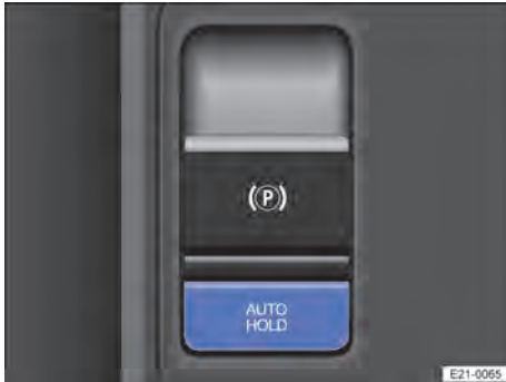
Fig. 128 In the centre console: button for Auto Hold.
