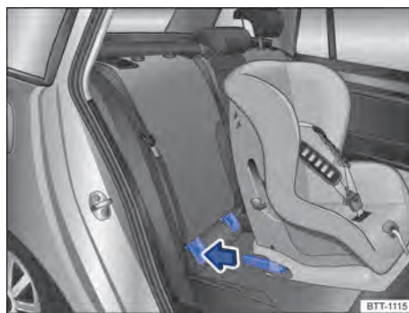
Fig. 44 Illustration: fitting an ISOFIX child seat with the attachment arms.
