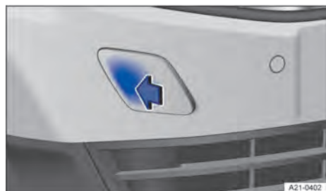
Fig. 199 In the front right bumper: Remove the cover.
