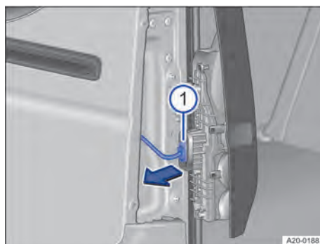
Fig. 187 On the tail lamp cluster: disconnecting the connector.
