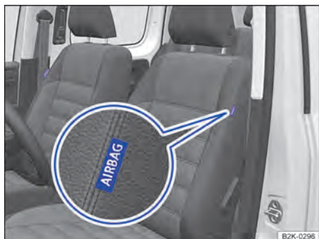
Fig. 34 On the side of the front seat: Location of the side airbag.
