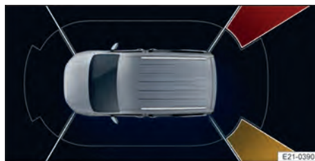
Fig. 139 On the Infotainment system screen: Cross Traffic Alert display.
